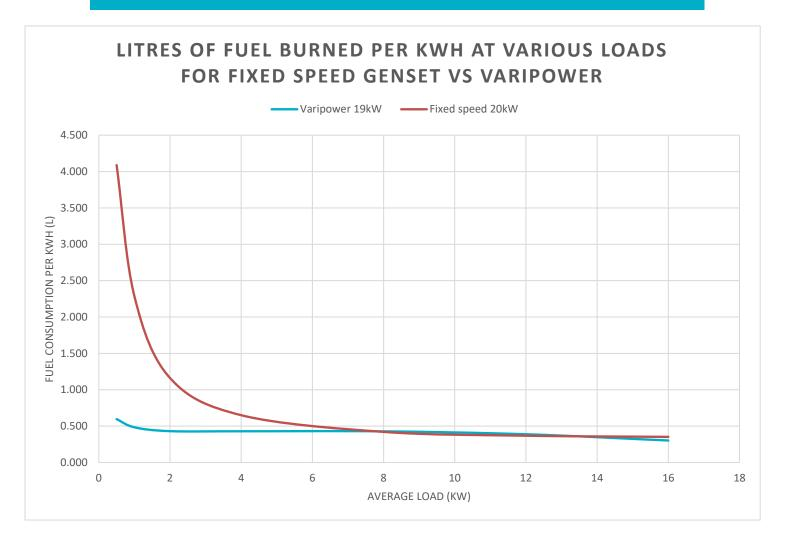
The graph illustrates how much fuel is burnt, by both a fixed speed 20kW generator and a 19kW VariPower, to supply power for different average loads.
