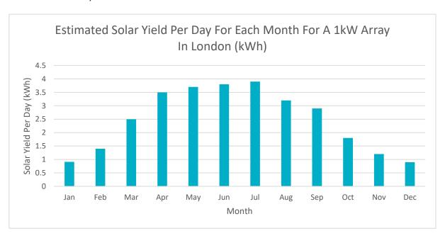
Taking the estimated solar yield data from the year, we get an average estimated daily yield of 2.5kWh for a 1kW array in London. This equates to an average of 100W solar yield per hour per 1kW of solar.
