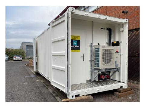
Overall the system, which was built at Energy's headquarters in Rochester, Kent, is designed to work autonomously - providing power from the solar panels and battery storage system until such time the demand exceeds the availability. When this happens, the system starts the generator automatically to provide power to the site at the same time recharging the batteries. The system ensures optimum performance at all times with a focus on using solar power ahead of generator power.
