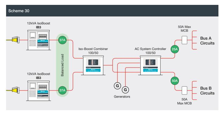
Allows for 2 x 240 volt shore cords (2 x 50 amp) and a 24 kVA generator and 12 kVA generator.
