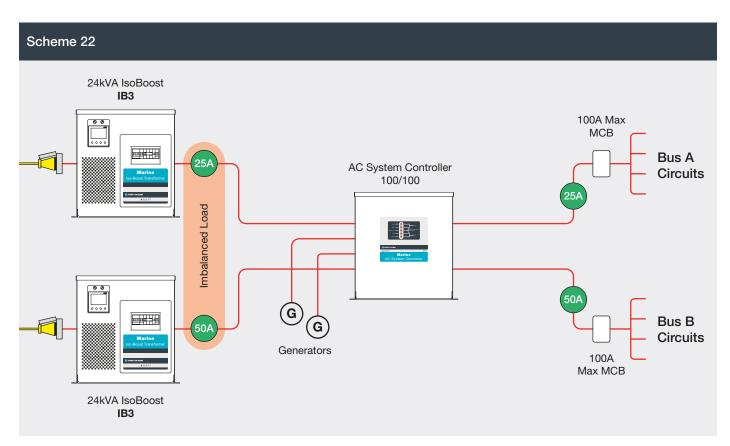
Allows for 2 x 240 volt shore cords (2 x 100 amp) and a 2 x 24 kVA generator. Twin shore-cords supply one output bus each. Mismatched bus loads cause mismatched shore supplies.
