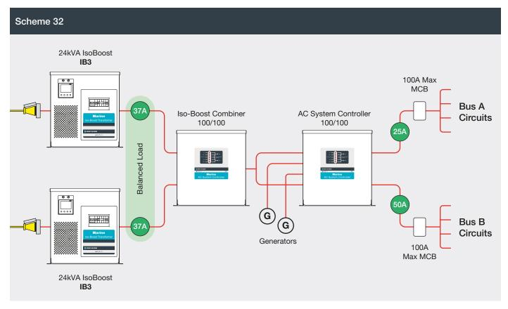
Allows for 2 x 240 volt shore cords (2 x 100 amp) and a 2 x 24 kVA generator.
