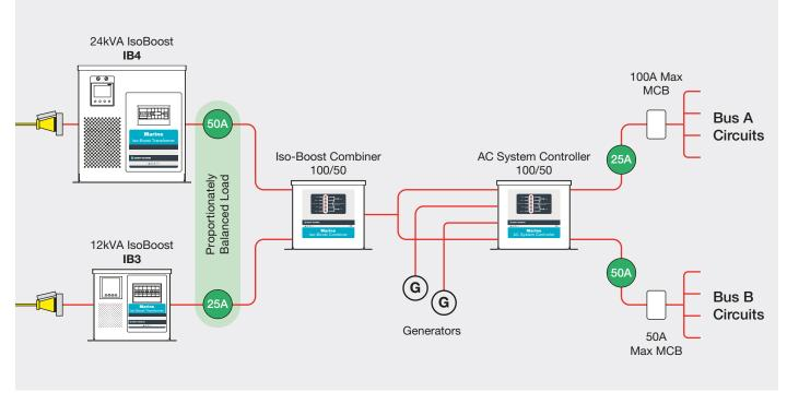
Allows for  $2 \times 240$  volt shore cords ( $1 \times 100$  amp and  $1 \times 50$  amp) and a 24 kVA generator and 12 kVA generator. Twin shore-cords combine to supply the ships load. Mismatched bus loads are balanced 66/33 across the shore supplies.
