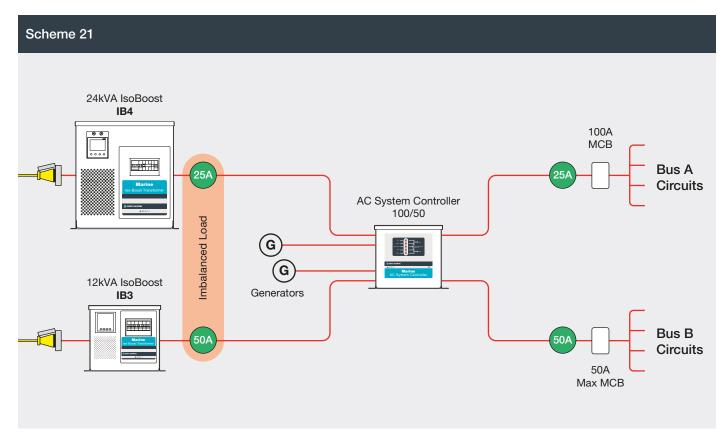
Allows for  $2 \times 240$  volt shore cords (1 x 100 amp and 1 x 50 amp) and a 24 kVA generator and 12 kVA generator. Twin shore-cords supply one output bus each. Mismatched bus loads cause mismatched shore supplies.
