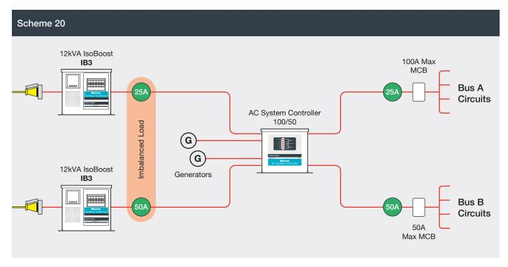
Allows for 2 x 240 volt shore cords (2 x 50 amp) and a 24 kVA generator and 12 kVA generator. Twin shore-cords supply one output bus each. Mismatched bus loads cause mismatched shore supplies.
