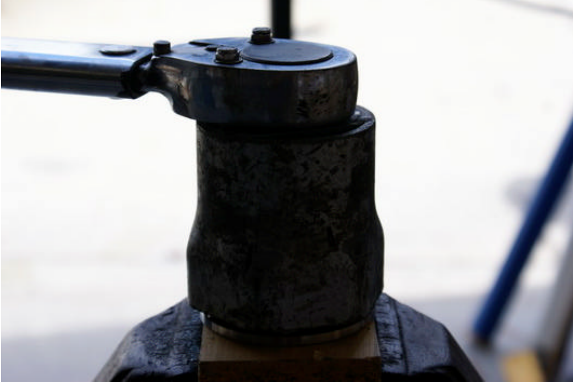
Housing set up in vise on \frac{3}{4} in timber block
